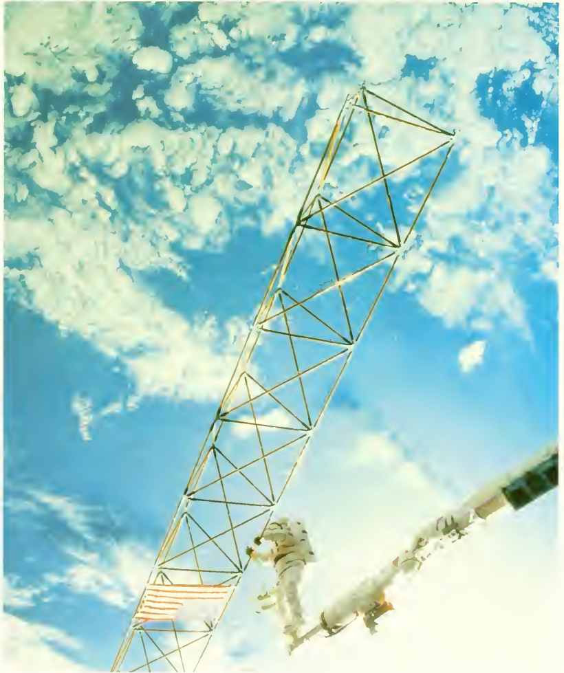
Astronaut Sherwood C. Spring, positioned on the end of the remote manipulator arm, checks joints on the assembly concept for construction of an erectable space structure tower. The tower in the photograph extends from the cargo bay of the Space Shuttle Atlantis.
